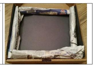
**Step 6:** Place the food you would like to cook/reheat in the solar oven and close the lid. (You can place an oven/meat thermometer in the solar oven during this step if you are interested in the internal temperature as you cook)
